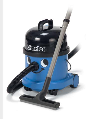
Powerful 1.6 Hp vacuum motor with 2 year warranty providing excellent dry soil or water recoveryMotor provides 110" waterlift and 95 CFM of airflowExcellent 0.5 micron filtration at 98.70 % efficiency for improved Indoor Air Quality with or without bagsWet or dry operation in a compact, powerful unitHandy carrying handle for dumpingBall float wet shut-off assembly ensures water does not reach the motorPolypropylene tanks for maximum durability and mobility
