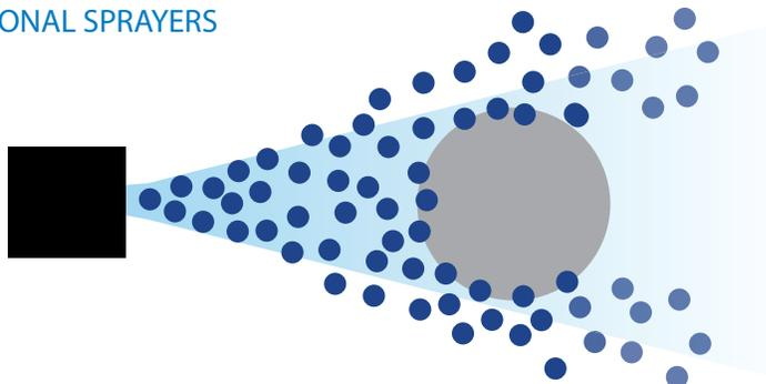
The Victory Series provide a fast and efficient application of chemicals. When the charged particles reach the desired surface, they uniformly disperse the product. The particles subsequently maintain their cationic charges for approximately 2 to 3 seconds – thus preventing grouting. This allows the solution to cover hidden and shaded areas, and also allows the user to cover a large area in a limited time.
