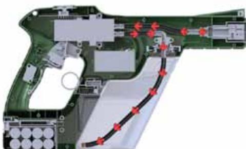
When the device is turned on, the charge begins at the charging ring and is transmitted in the unit, to the pump and the tank – thus charging all positive ions.
